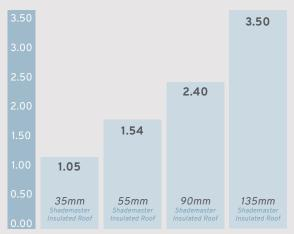
All calculations for the above are based on a mean temperature of 23°C in compliance with AS 4859.1:2002 Section 2.3.3.3
